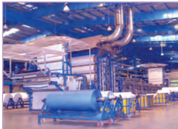
Pad steam dyeing range-versatile fabric processing machine with advance dyeing features
