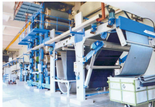
Combo Desizer cum Merceriser Machine - Advanced Denim Fabric Processing Machine with combination of Desizing, Mercerising and Dyeing range
