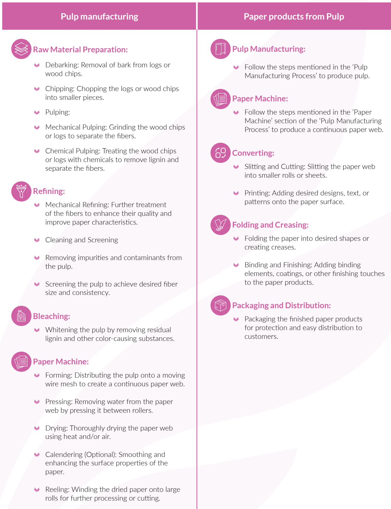
Diagram – Pulp and Paper Products from Pulp – Manufacturing Process
